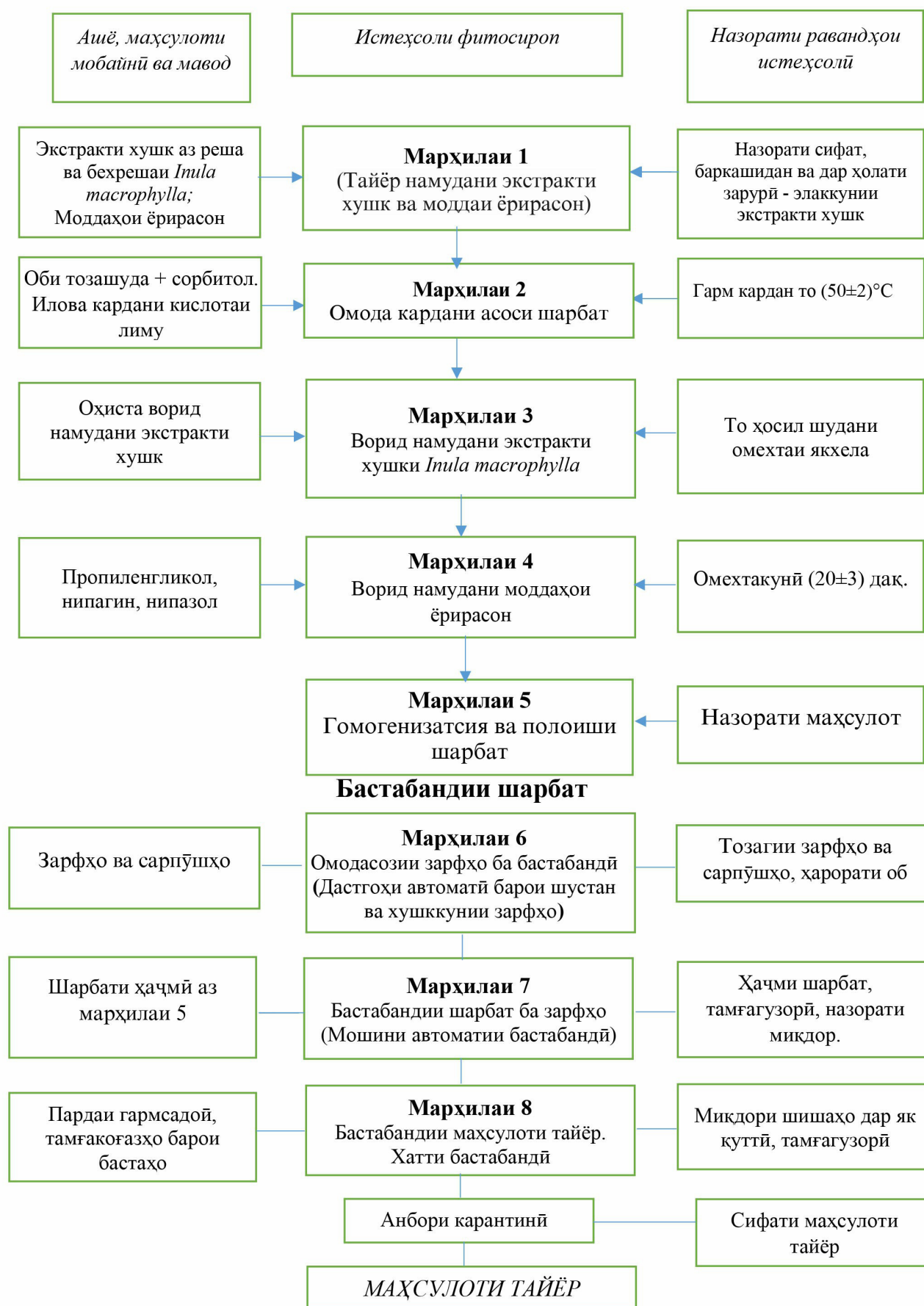
Расми 7. Нақшаи технологии истеҳсоли «Инуланта» Figure 7. Process flow diagram for the production of "Inulanto"
